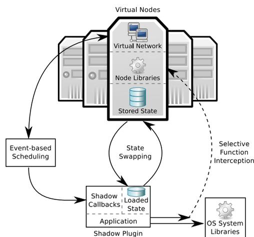
Figure 1: Shadow’s architectural design. Using a plug-in wrapper, real-world applications are integrated into Shadow as virtual nodes while system and library calls are intercepted and replaced with Shadow-specific implementations.
