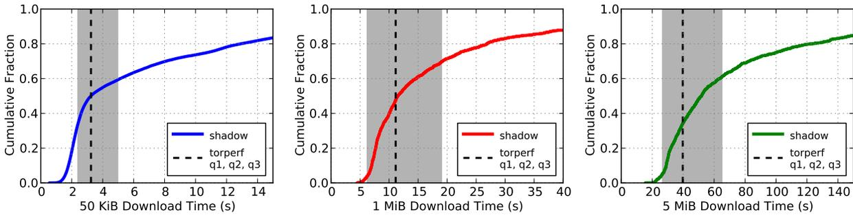
Figure 4: Shadow-Tor compared with live-Tor network performance. TorPerf represents statistics from [metrics.torproject.org](https://metrics.torproject.org). The gray area shows TorPerf first to third quartile stretch while the dotted line represents the TorPerf median. Shadow closely approximates Tor performance for all file sizes.
