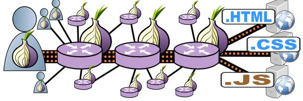
Figure 1: Connections between Tor clients, relays, and destinations. Solid black lines represent TCP connections, and dashed orange lines represent logical streams of client application payloads that are multiplexed over both the TCP connections and the encrypted circuits that are constructed by clients. High performance relays generally maintain thousands of open network sockets as a result of this architecture.
